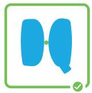
Distance between convex contours needs a distance of 0.3mm
